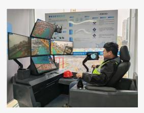
Swire Properties is pioneering the use of a Remote Control Tower Crane system in Taikoo Li Xi'an, a significant advancement in construction safety and efficiency. By positioning the crane operator on the ground and employing AI technology, this system eliminates the need for crane operators to ascend the tower, thereby removing a crucial safety hazard. Instead, operators control the crane from a secure onsite cabin.
